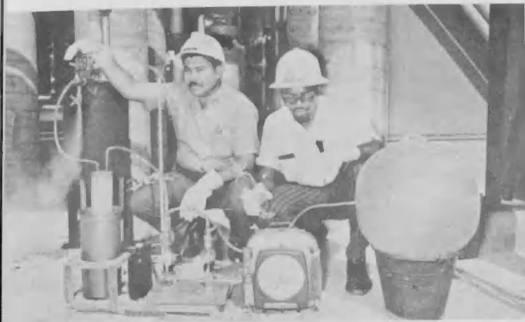
Assistant Juan Ras (left) and Chemist Pedrito Cornett take pentane gas sample at the Hydrogen Unit for testing for sulfur in the 0.5 ppm range, for hydrogen sulfide and hydrocarbons in the feed gas.
